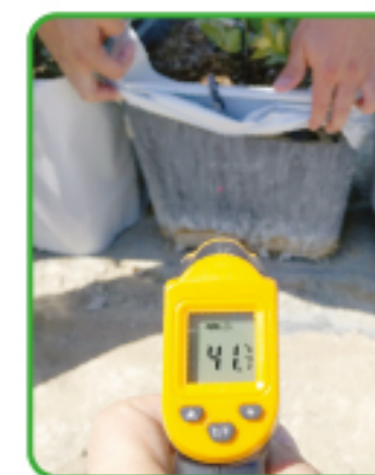
Pot temperature with cooling skirt raised.
