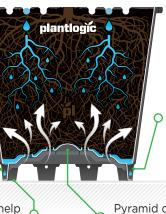
Legs connected to edge holes breaks drainage surface tension eliminating saturated zone.
